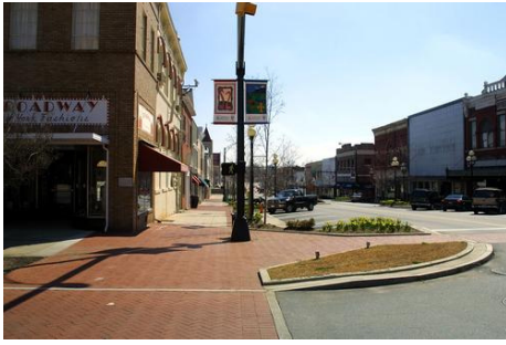
A Well-Designed Streetscape, Like this One in Anderson, South Carolina, Including Brick Crosswalks, Landscaped “Neck-Downs”, and Diagonal Parking, is Proposed for Highland Avenue (from www.contextsensitivesolutions.org )
