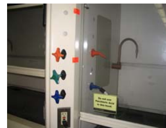
Note orange sash height marks.
